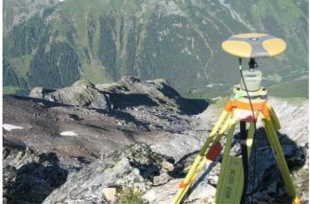
A photograph showing a surveying instrument, likely a total station or GNSS receiver, mounted on a yellow tripod. The instrument is positioned on a rocky, mountainous terrain with a valley and mountains in the background. | Falaises et glissements de terrain | Lieu : Valais et Vaud | Surveillances de falaises par mesures GPS et terrestres combinées<br>Compensation globale du réseau<br><br>Précision <1cm |
